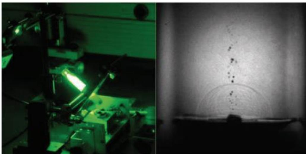
**Figure 6 Photographs showing laser ablation in a liquid. The photographs provided by Dr. Takeshi Tsuji, Kyushu University, Japan.**
