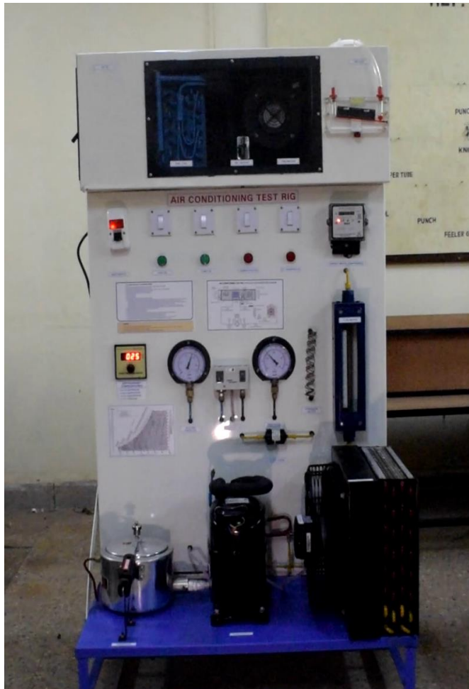
Experimental Air Conditioning tutor with AHU.
