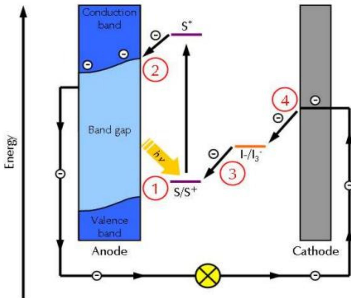
**Figure 1.4 Mechanism of dye-sensitized solar cell**
