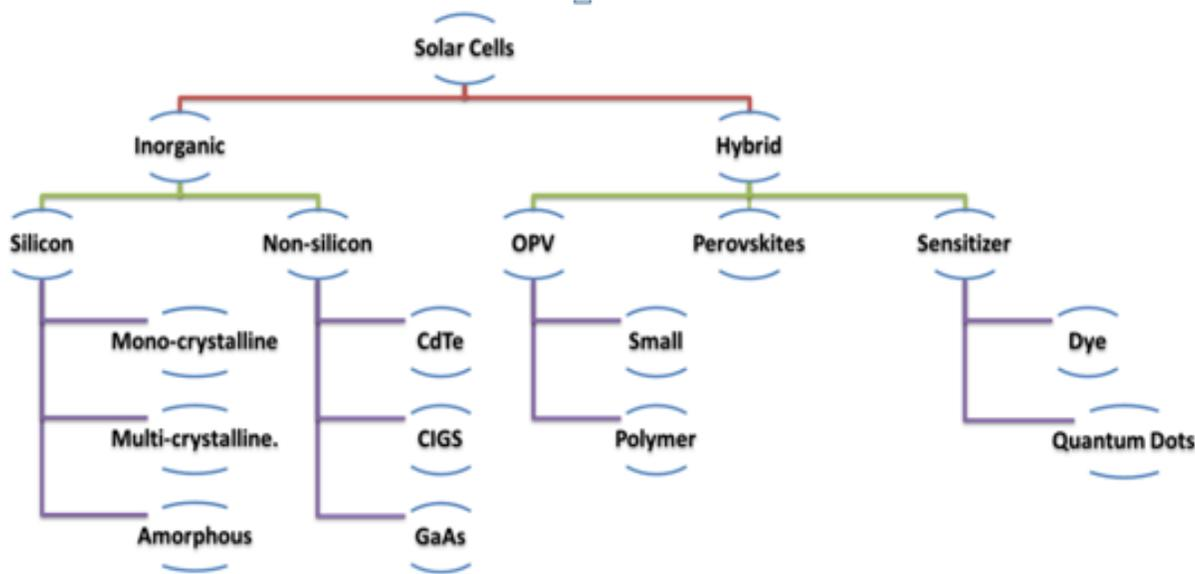
**Figure 1.1 Classification of photovoltaic technology**
