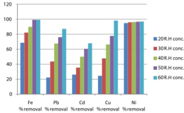
**Fig. 4 The husk of rice is an efficient solvent for removing several heavy metals.**
