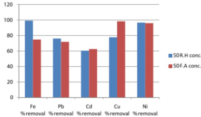
**Fig. 7** When the adsorbent concentration was 50 mg/l, a comparison was made between the removal effectiveness of rice husk and fly ash.
