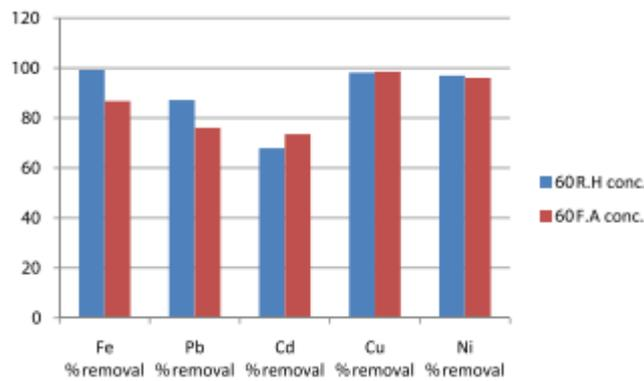
**Fig. 6 Comparative analysis of the removal effectiveness of rice husk and fly ash at an absorbent concentration of sixty milligrammes per litre.**
