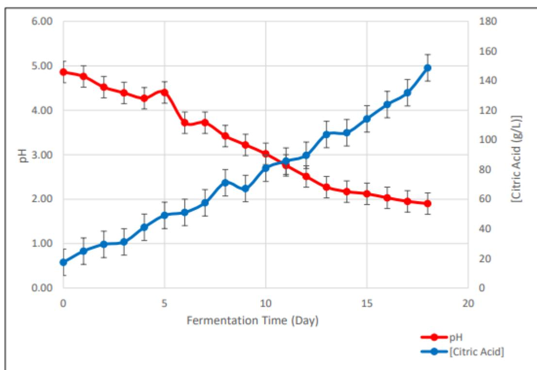
Figure 1. Profile of citric acid concentration and pH value during fermentation.
