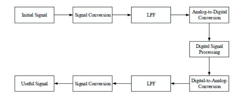
**Figure-1 : Digital Signal Processing flow**
