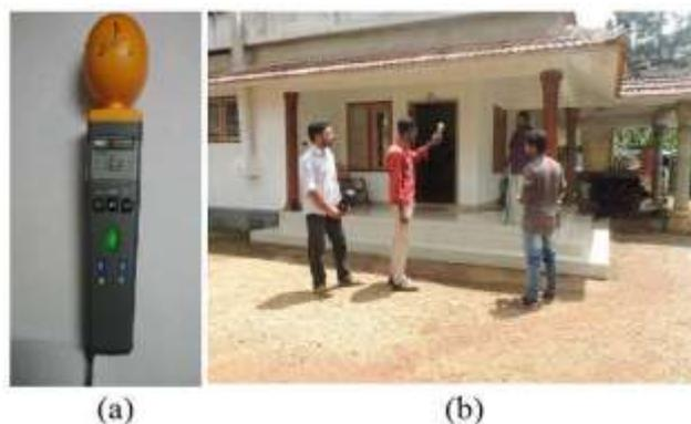
**Figure 1: (a) Photograph of the MECO's Electrosmog Meter 9720 and (b) its usage.**
